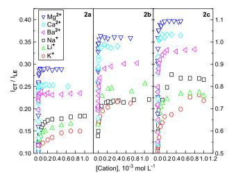
Figure 5. Plots of the CT to LE fluorescence intensity ratios of **2a**–**c** versus cation concentration. Plots of **2a** have the left coordinate and those of **2b** and **2c** have the same right coordinate.
