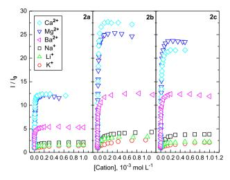
**Figure 3.** The CT fluorescence intensity enhancement ( $III_0$ ) of **2a-c** as a function of cation concentration. Excitation wavelength was 300 nm. I and  $I_0$  represent the CT emission intensities in the presence and absence of the metal cation, respectively.
