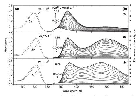
Figure 2. Absorption (a) and fluorescence spectra (b) of  $2a (1.00 \times 10^{-5} \text{ mol L}^{-1})$ ,  $2b (1.22 \times 10^{-5} \text{ mol L}^{-1})$ , and  $2c (1.00 \times 10^{-5} \text{ mol L}^{-1})$  in ACN in the absence and the presence of excess amount of  $Ca^{2+}$  (a) and of increasing concentration of  $Ca^{2+}$  (b). All metal cations existed in the form of perchlorate. Excitation wavelength was 300 nm. Asterisks in (b) refer to Raman scattering.
