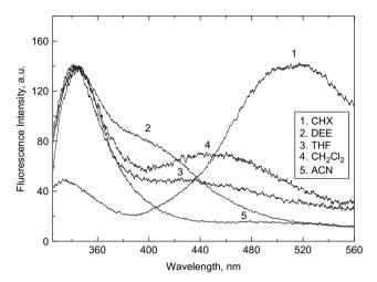
**Figure 1**. Fluorescence spectra of **2a** in solvents of varied polarity. Solvent: CHX, cyclohexane; DEE, diethyl ether; THF, tetrahydrofuran; CH<sub>2</sub>Cl<sub>2</sub>, dichloromethane; and ACN, acetonitrile. [**2a**]= $1.00\times10^{-5}$  mol L<sup>-1</sup>. Excitation wavelength was 290 nm.
